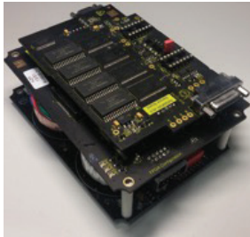
RadMon V6 radiation monitoring system and CELESTA CubeSat payload test board
