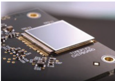
Timepix3 chip (multipurpose hybrid pixel detector developed within the Medipix3 Collaborations) and Timepix-based radiation detector (SATRAM) aboard Proba-V
